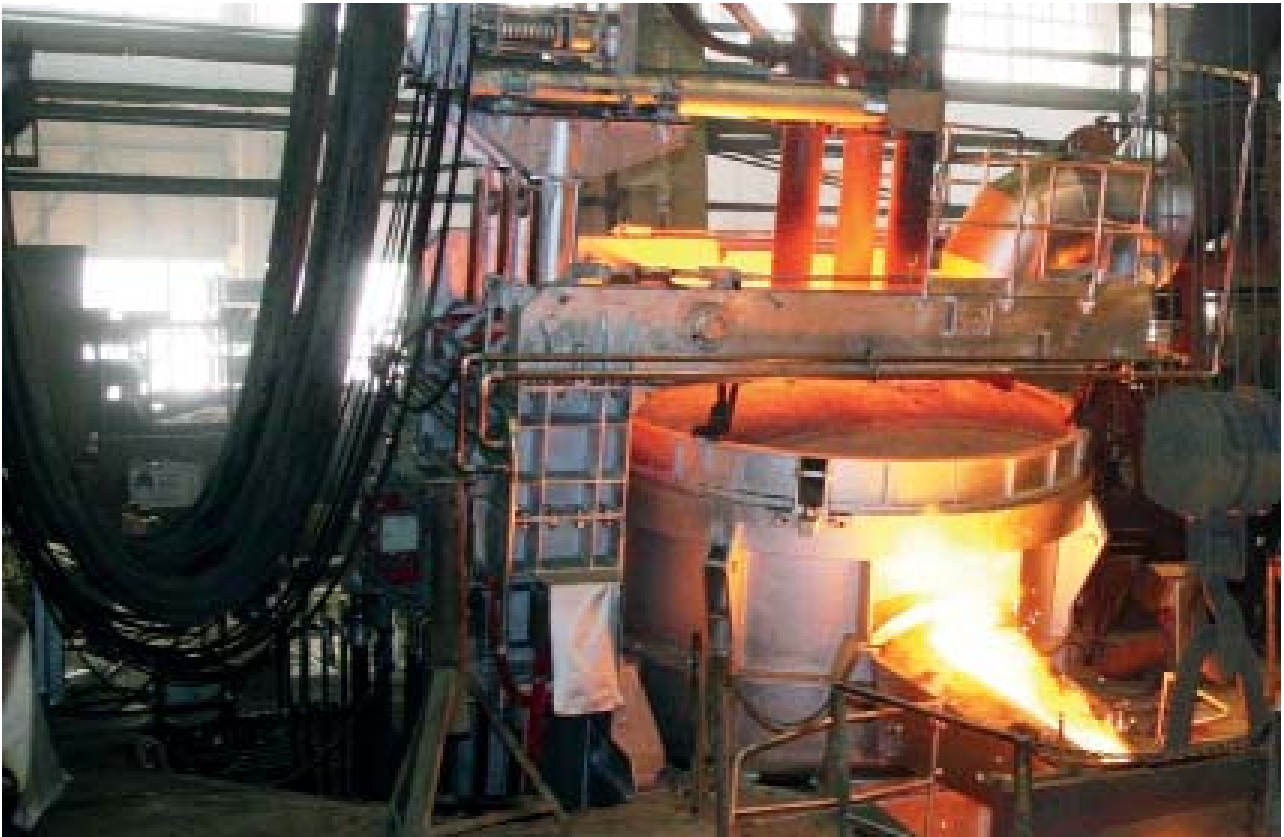
Overhauled electric arc furnace during tapping (Photos: SHB )
